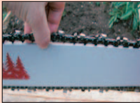
Chain won't turn? Check to make sure the chain tension is set correctly.
