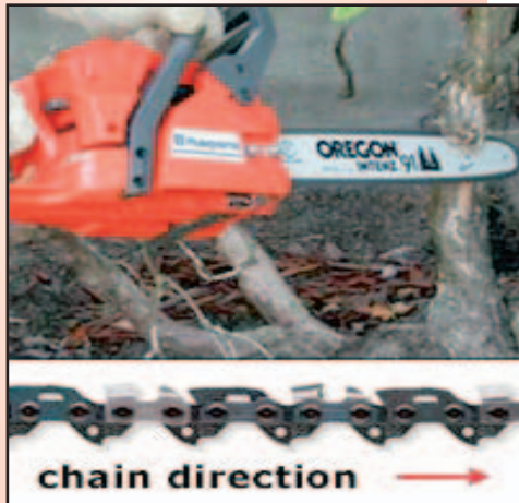
The front of your chain's cutters should always face and drive towards the tip of your bar.
